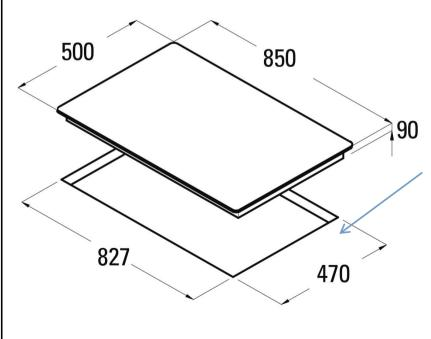
Cut 4 corners must be in round to avoid table tap cracking
